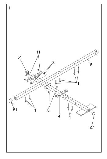
Slide the Assist Upright (74) and the Leg Press Upright (56) onto the indicated 5/16" x 2 1/2" Carriage Bolts (1) in the Stabilizer (5). The high side of the brackets on the Uprights should be on the side shown. Hand-tighten four 5/16" Nylon Locknuts (3) onto the Carriage Bolts. Do not tighten the Nylon Locknuts yet.
